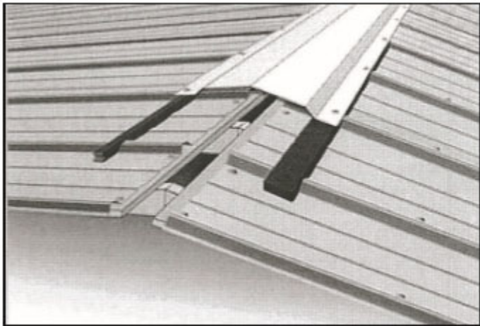
Ridge cap showing outside closure and profile vent.
