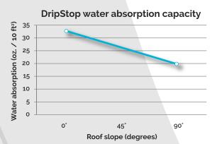
The bond holding the water is so strong, that even at forty-five degree slope it still holds 26 ounces of moisture! DripStop can hold more than one quart of water per ten square feet of roof space.
