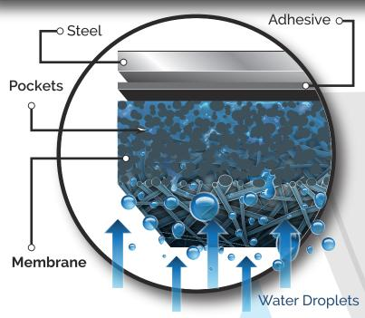
When climate conditions cause condensation to occur, DripStop absorbs and holds that moisture in specially designed pockets in the membrane. When climate conditions go back above the dew point, the moisture is released back into the air as normal humidity.
